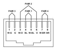
Figure 6-2. RJ-45 connector using T568A wiring.
